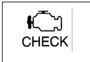
Your vehicle is equipped with a computer that monitors the operation of the LPG fuel system. If the computer detects a specific emission system problem, the CHECK ENGINE light will come on. Your vehicle may require service. See “Malfunction Indicator Lamp” in the Index of your GM owner’s manual.
