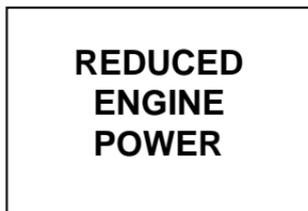
If the engine coolant temperature is below freezing (32°F (0°C)), the REDUCED ENGINE POWER light will come on. In this mode, the engine speed will not go above idle, even if you press the accelerator pedal. The light will stay on and the engine will operate in this mode until the engine coolant temperature reaches 32°F (0°C). You can then drive your vehicle as normal.
