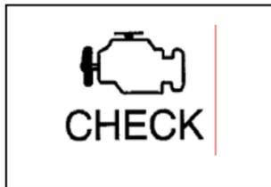
Your vehicle is equipped with a computer that monitors the operation of the propane fuel system. If the computer detects a fuel system problem, the CHECK ENGINE light will come on. Your vehicle may require service. See “Malfunction Indicator Lamp” in the Index of your GM owner’s manual.
